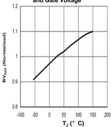
Figure 6: Break Down vs. Junction Temperature
