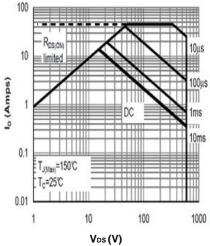
Figure 11: Maximum Forward Biased Safe Operating Area
