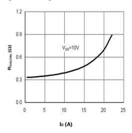
Figure 4: On-Resistance vs. Drain Current and Gate Voltage
