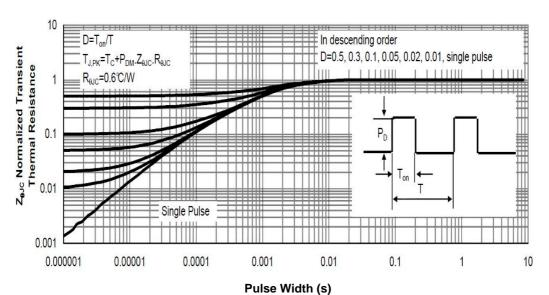
Figure 12: Normalized Maximum Transient Thermal Impedance
