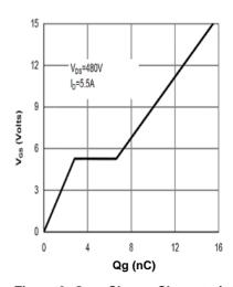
Figure 8: Gate-Charge Characteristics
