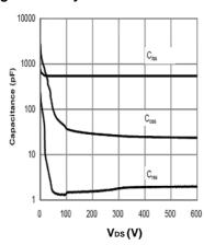
Figure 9: Capacitance Characteristics
