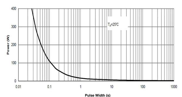
Figure 15: Single Pulse Power Rating Junction-Ambient
