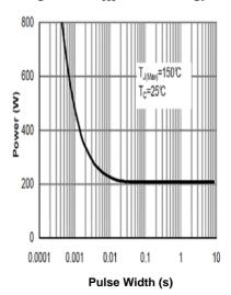
Figure 12: Single Pulse Power Rating Junction to Case
