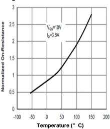
Figure 5: On-Resistance vs. Junction Temperature
